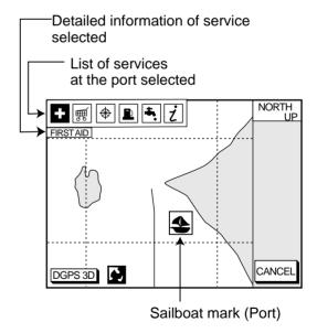
Figure 3-8 Plotter display showing Nav-Charts™ port service display
